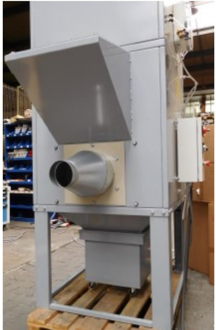
Pressure relief flap of the extraction for aluminium dust
