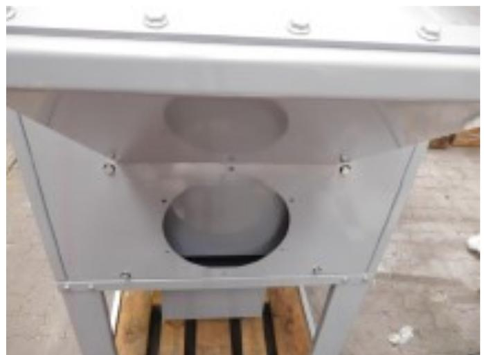
Internal spark baffle
